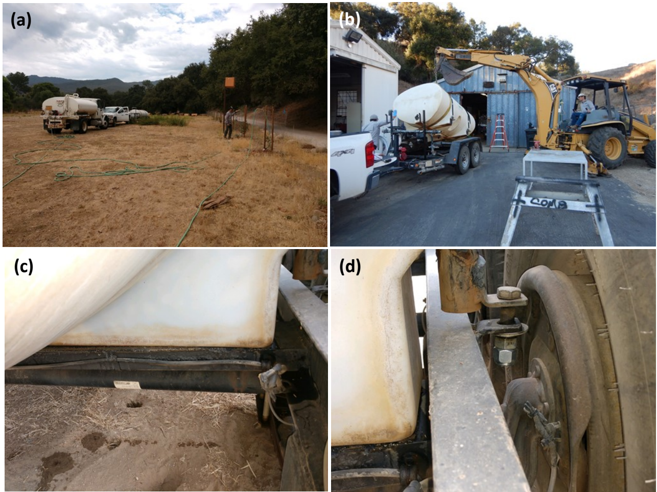
Exhibit 1: Watering Year 13 oak trees at Live Oak Camp using both COMB watering rigs (a) and repairing the water trailer first lifting up the tank (b), repositioning and regluing the carpet cushion between the tank and the trailer frame (c), and double nutting the bolts that attach the tank to the trailer with lock nuts (d).
