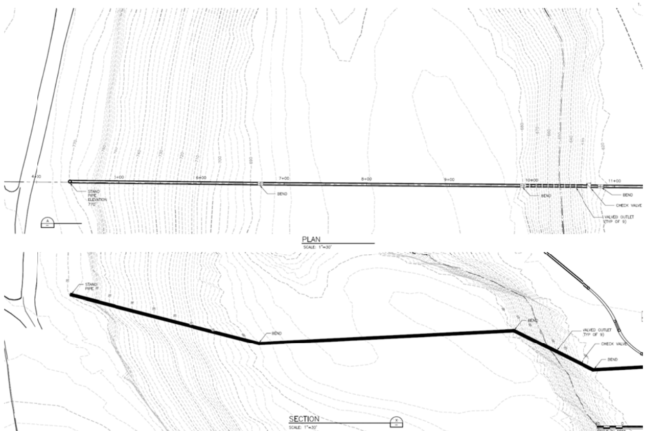
Figure 9. Standpipe recommended for surge protection. This pipeline is not needed for the shore-mounted PS.
