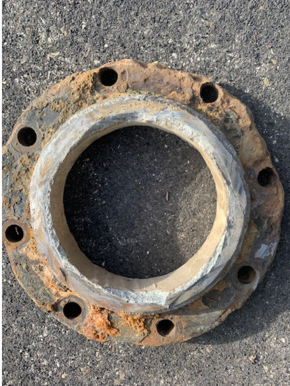
Corroded Steel Flange on SCC Outlet
