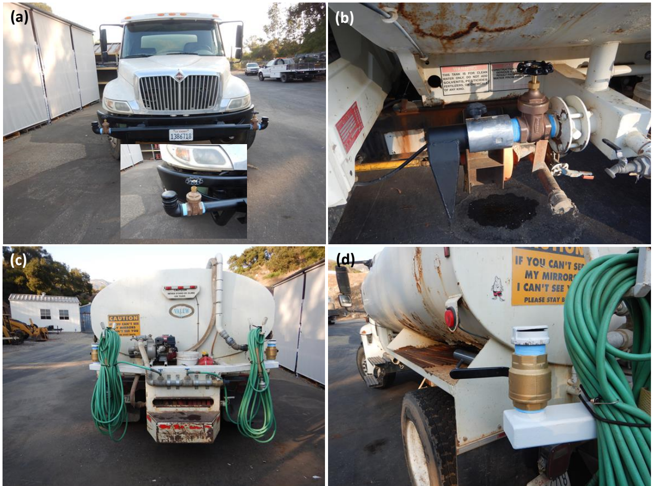
Exhibit 1: Lake Cachuma Oak Tree Restoration program showing newly installed (a) front, (b) side, and rear shutoff valves on the large sprayers.
