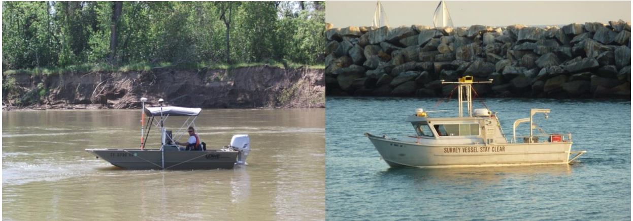
Figure 2: Fugro’s Survey Skiff acquiring Single-beam Echosounder Data, and the M/V Julie Ann acquiring Multibeam Data.
