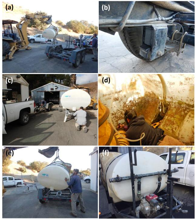
**Exhibit 1:** Water trailer maintenance showing (a) removal of tank, (b) new suspension welds, plastic welding (c) outside of the tank and (d) inside of the tank, (e) placing the tank on top of new trailer carpet, and (f) new hose and pipe connectors.
