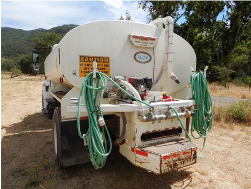
Figure 21: Water tanker truck with newly installed Honda pump motor on rear.
