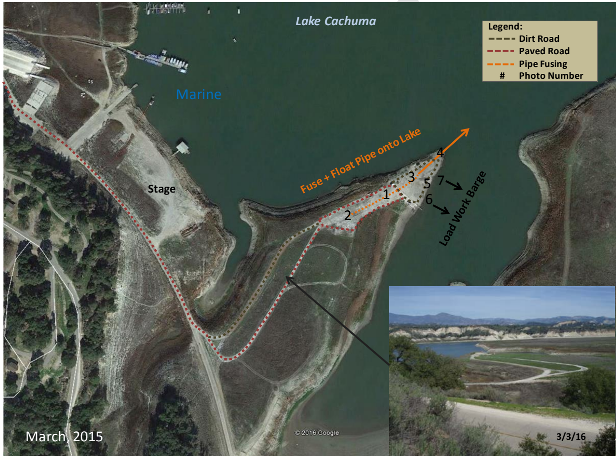
Figure 5: Access via asphalt and dirt roads to the staging area, Transmission Pipe fusing location and direction to float it onto the lake, and boat ramps for loading Anchor Piles onto the construction barge; numbers are photos presented in Figures 6 and 8.
