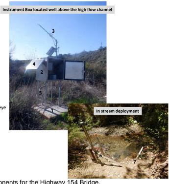
Exhibit 3: Proposed USGS gauging station components for the Highway 154 Bridge.
