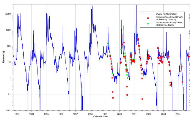
Figure 2-13. Daily flow hydrograph for USGS Gage at Lompoc Narrows (ID No. 11133000) and other flow measurements (Source: USGS 2005; CPWA 2005; Stetson 2005)
