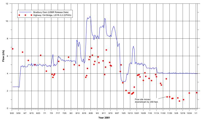
Figure 2-15. Hydrograph of releases at Bradbury Dam and flow measurements in the Santa Ynez River at Highway 154 Bridge (Source: Reclamation 2005; CPWA 2005; Stetson 2005)
