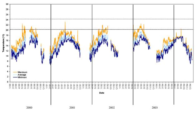
Figure 3-38. Quiota Creek (QC-2.71) water temperatures, 2000 – 2004 (Note: Data gaps in the temperature record are the result of removing units during the winter, unit dewatering, or instrument failure (Source: CPWA 2005))
