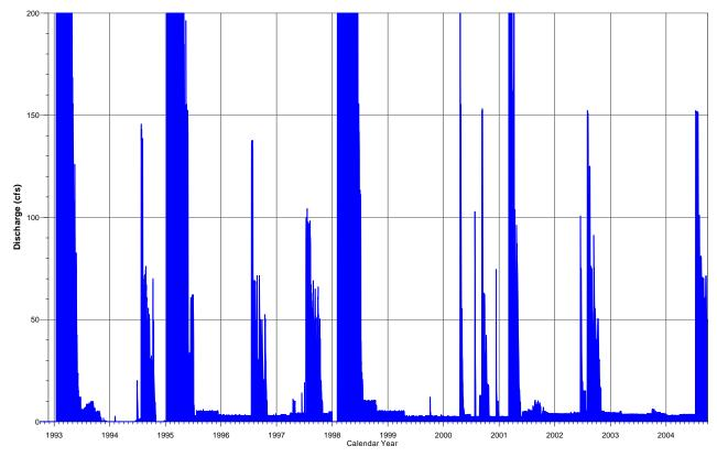
Figure 2-6. Daily discharge from Lake Cachuma shown on linear scale (not including leakage; Source: CPWA 2005; Stetson 2005)
