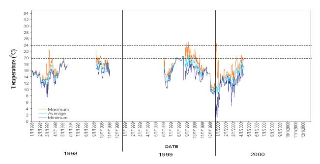
Figure 3-27. 1998 – 2000 Santa Ynez River water temperatures, Santa Ynez Lagoon at Ocean Park (LSYR-47.75), Bottom Unit 6 feet below surface (Note: Data gaps in the temperature record are the result of removing units during the winter, unit dewatering, or instrument failure (Source: CPWA 2005))
