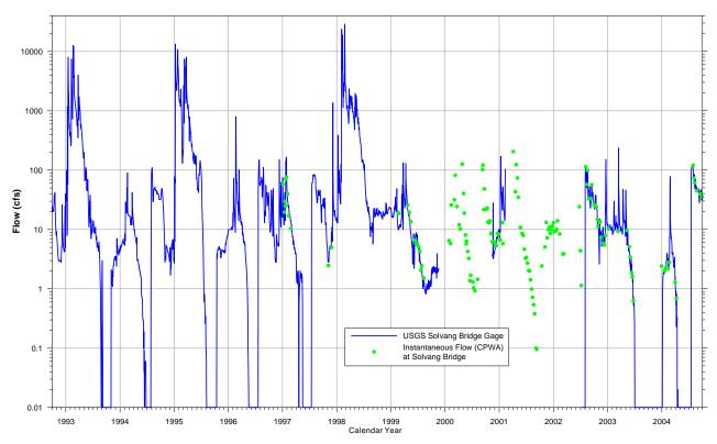
Figure 2-12. Daily flow hydrograph for USGS Gage at Solvang Bridge (ID No. 1112850) and other flow measurements (Source: USGS 2005, CPWA 2005, and Stetson 2005)
