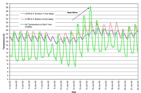
Figure 3-2. Example of Effects of Diel Air Temperatures on Water Temperatures at Pool Located at the Lower Gainey Crossing, LSYR-6.4 (Source: CPWA 2005, Stetson 2008)
