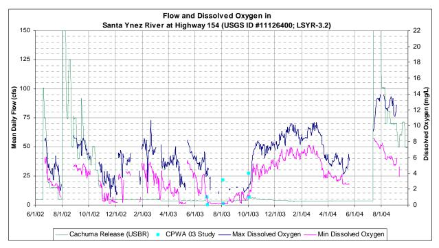
Figure 3-32. USGS Flow and DO Concentration Measurements in Santa Ynez River at Highway 154 Bridge, LSYR-3.2 (Source: USGS 2008, Stetson 2008, CPWA 2005)
