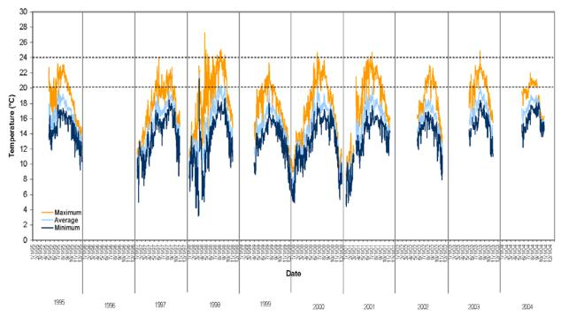
Figure 3-41. Upper Salsipuedes Creek (SC-3.8) water temperatures, 1995 – 2004 measured 3.8 miles upstream of the Santa Ynez river confluence-50 feet upstream of El Jaro confluence (Note: Data gaps in the temperature record are the result of removing units during the winter, unit dewatering, or instrument failure (Source: CPWA 2004))
