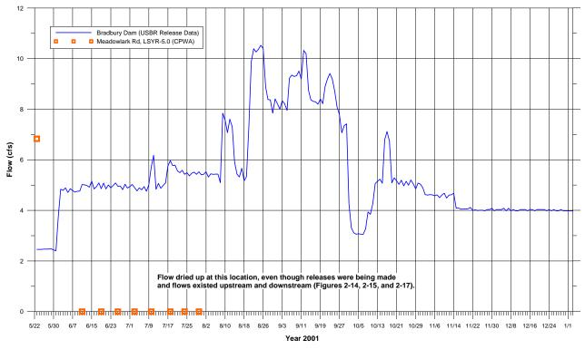
Figure 2-16. Hydrograph of releases at Bradbury Dam and flow measurements in the Santa Ynez River at Meadowlark Road (Source: Reclamation 2005; CPWA 2005; Stetson 2005)
