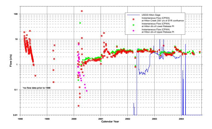
Figure 2-19. Daily flow hydrograph for USGS Gage in Hilton Creek (ID No. 11125600) and other flow measurements (note: HCWS began in April 2000; Source: USGS 2005, Stetson 2005; CPWA 2005)
