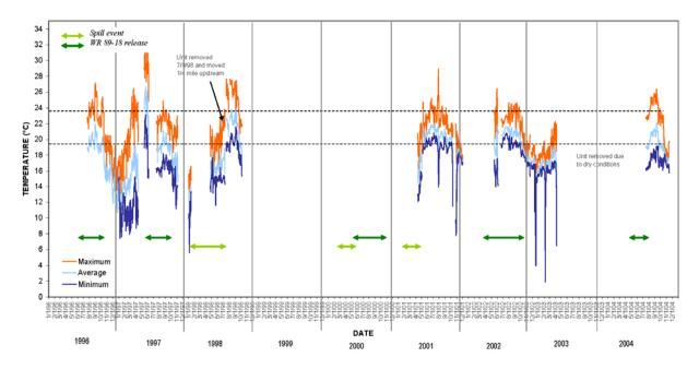
Figure 3-20. 1995 – 2004 Santa Ynez River water temperatures, Refugio Reach (LSYR-5.0), 5.0 miles downstream of Bradbury Dam, Bottom Unit (Note: Data gaps in the temperature record are the result of removing units during the winter, unit dewatering, or instrument failure. No monitoring was performed between 1999 and mid-2001. (Source: CPWA 2005))
