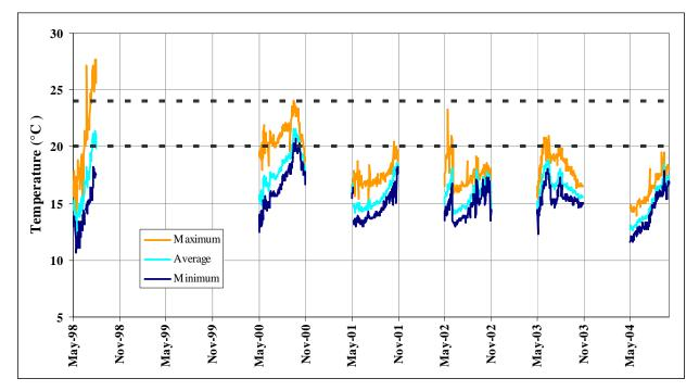
Figure 3-37. Lower Hilton Creek (HC-0.12) water temperatures, 1995 – 2004 (Note: Data gaps in the temperature record are the result of removing units during the winter, unit dewatering, or instrument failure (Source: CPWA 2005))
