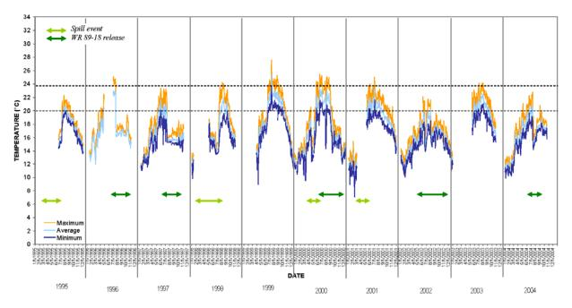
Figure 3-17. 1995 – 2004 Santa Ynez River water temperatures at Long Pool (LSYR-0.5), 0.5 miles downstream of Bradbury Dam, Surface Unit thermograph – 1 foot below surface (Note: Data gaps in the temperature record are the result of removing units during the winter, unit dewatering, or instrument failure (Source: CPWA 2005))
