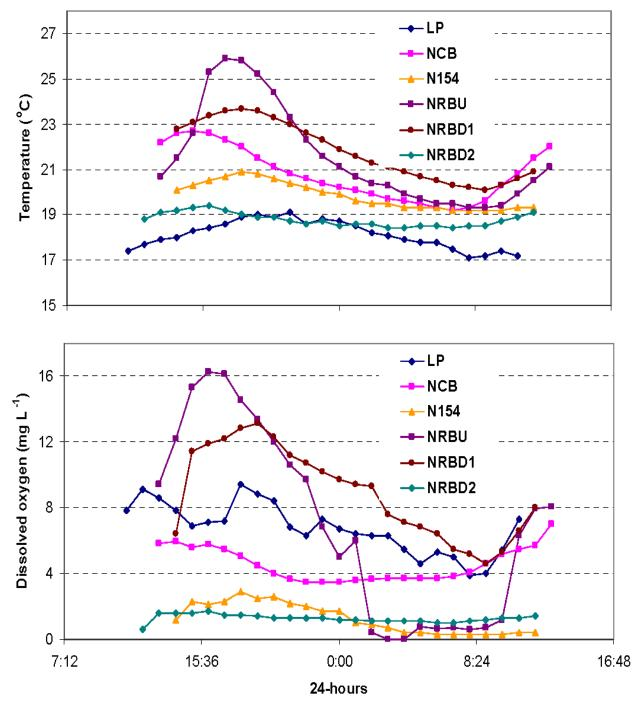
Figure 3-30. Pool water quality conditions, temperature and DO during August for all of the five to seven pools monitored on the mainstem of the Santa Ynez River during the summer of 2003 (See Figure 3-28 for pool locations (Source: CPWA 2005))
