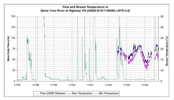
Figure 3-12. Flow and USGS Stream Temperature in Santa Ynez River at 154 Bridge, LSYR-3.2 (Source: USGS 2008, Stetson 2008)
