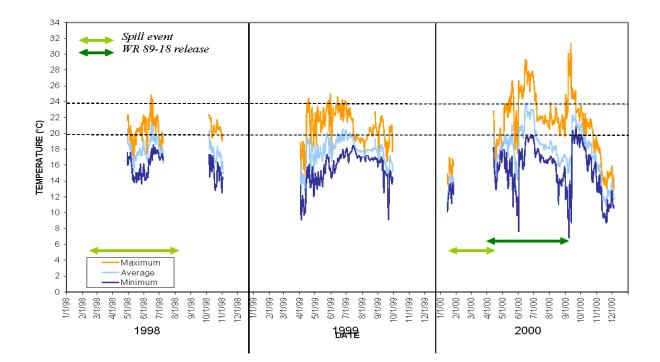
Figure 3-25. 1998 – 2000 Santa Ynez River water temperatures, Cargasacchi Reach, LSYR-22.45; Surface Unit, 1 foot below the surface; Note: Private landowner restricted access in 2000 which prevented further monitoring (Note: Data gaps in the temperature record are the result of removing units during the winter, unit dewatering, or instrument failure (Source: CPWA 2005))
