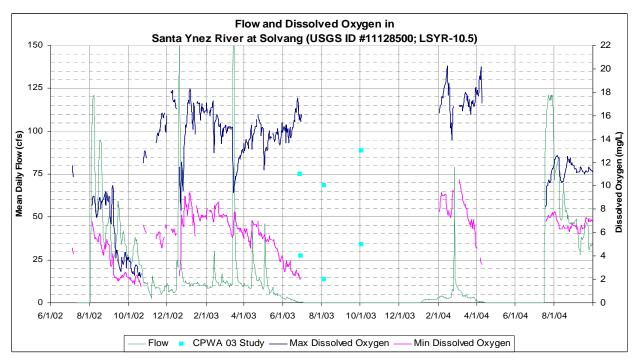
Figure 3-33. USGS Flow and DO Concentration Measurements in Santa Ynez River at Solvang, LSYR-10.5 (Source: USGS 2008, Stetson 2008, CPWA 2005)
