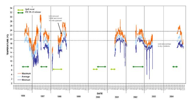
Figure 3-19. 1996 – 2004 Santa Ynez River water temperatures, Refugio Reach (LSYR-5.0), 5.0 miles downstream of Bradbury Dam, Surface Unit thermograph – 1 foot below surface (Note: Data gaps in the temperature record are the result of removing units during the winter, unit dewatering, or instrument failure. No monitoring was performed between 1999 and mid-2001. (Source: CPWA 2005))
