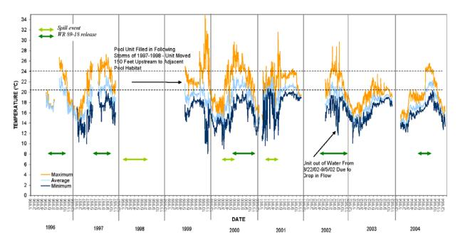
Figure 3-22. 1996 – 2004 Santa Ynez River water temperatures, Alisal Reach (LSYR-7.8), 7.8 miles downstream of Bradbury Dam, Bottom Unit, 4 feet below surface (Note: Data gaps in the temperature record are the result of removing units during the winter, unit dewatering, or instrument failure (Source: CPWA 2005))
