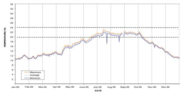
Figure 3-15. Water temperatures at the Stilling Basin (LSYR-0.2), 1999, at a depth of 3 feet (Note: This was exploratory monitoring that confirmed that water temperatures are not much different at this location than at the Long Pool (LSYR-0.5); Source: CPWA 2004)
