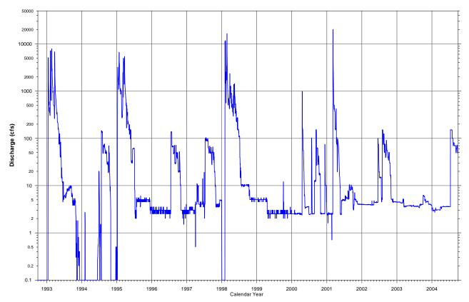
Figure 2-5. Daily discharge from Lake Cachuma shown on log scale (not including leakage; Source: CPWA 2005; Stetson 2005)
