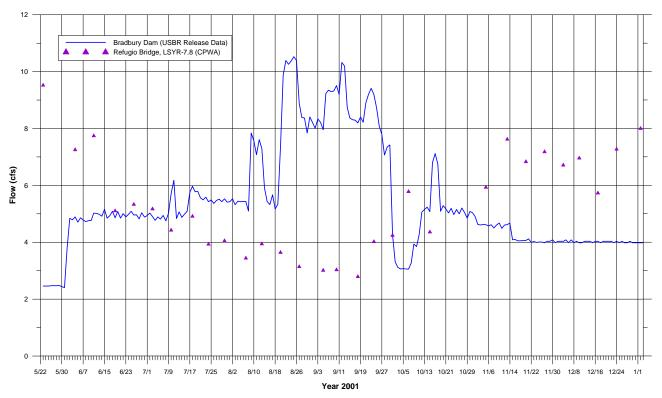
Figure 2-17. Hydrograph of releases at Bradbury Dam and flow measurements in Santa Ynez River at Refugio Bridge (Source: Reclamation 2005; CPWA 2005; Stetson 2005)
