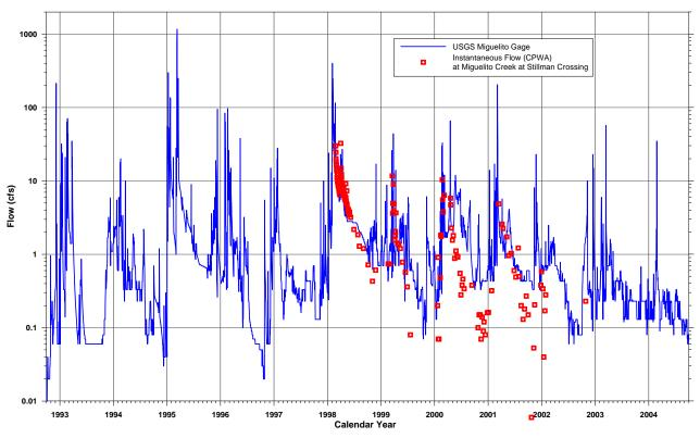
Figure 2-20. Daily flow hydrograph for USGS Gage in San Miguelito Creek (ID No. 11134800) and other flow measurements (Source: USGS 2005, Stetson 2005; CPWA 2005)
