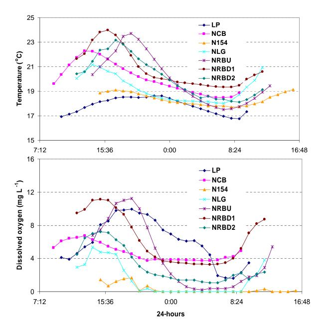
Figure 3-29. Pool water quality conditions, temperature and DO at the end of June for all of the seven pools monitored on the mainstem of the Santa Ynez River during the summer of 2003 (see Figure 3-28 for pool locations) Source: CPWA 2005))
