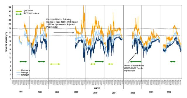
Figure 3-21. 1996 – 2004 Santa Ynez River water temperatures, Alisal Reach (LSYR-7.8), 7.8 miles downstream of Bradbury Dam, surface unit 1 foot below the surface (Note: Data gaps in the temperature record are the result of removing units during the winter, unit dewatering, or instrument failure (Source: CPWA 2005))
