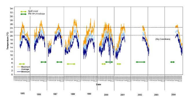
Figure 3-24. 1995 – 2004 Santa Ynez River water temperatures, Buellton Reach at Avenue of the Flags Bridge (LSYR-13.9), 13.9 miles downstream of Bradbury Dam (Note: Data gaps in the temperature record are the result of removing units during the winter, unit dewatering, or instrument failure (Source: CPWA 2005))
