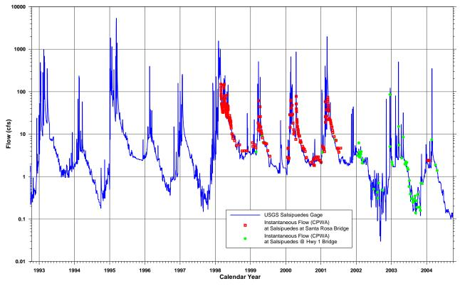
Figure 2-18. Daily flow hydrograph for USGS Gage in Salsipuedes Creek (ID No. 11132500) and other flow measurements (Source: USGS 2005, Stetson 2005; CPWA 2005)
