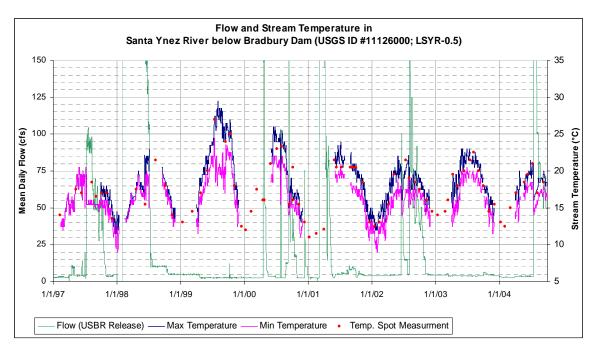
Figure 3-11. Flow and USGS Stream Temperature in Santa Ynez River below Bradbury Dam; LSYR-0.5 (Source: USGS 2008, Stetson 2008)
