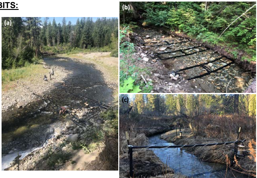
Exhibit 1: Examples of PIT tagging operations: (a) 30 foot swim over, (b) 15 foot swim over, and (c) swim through.
