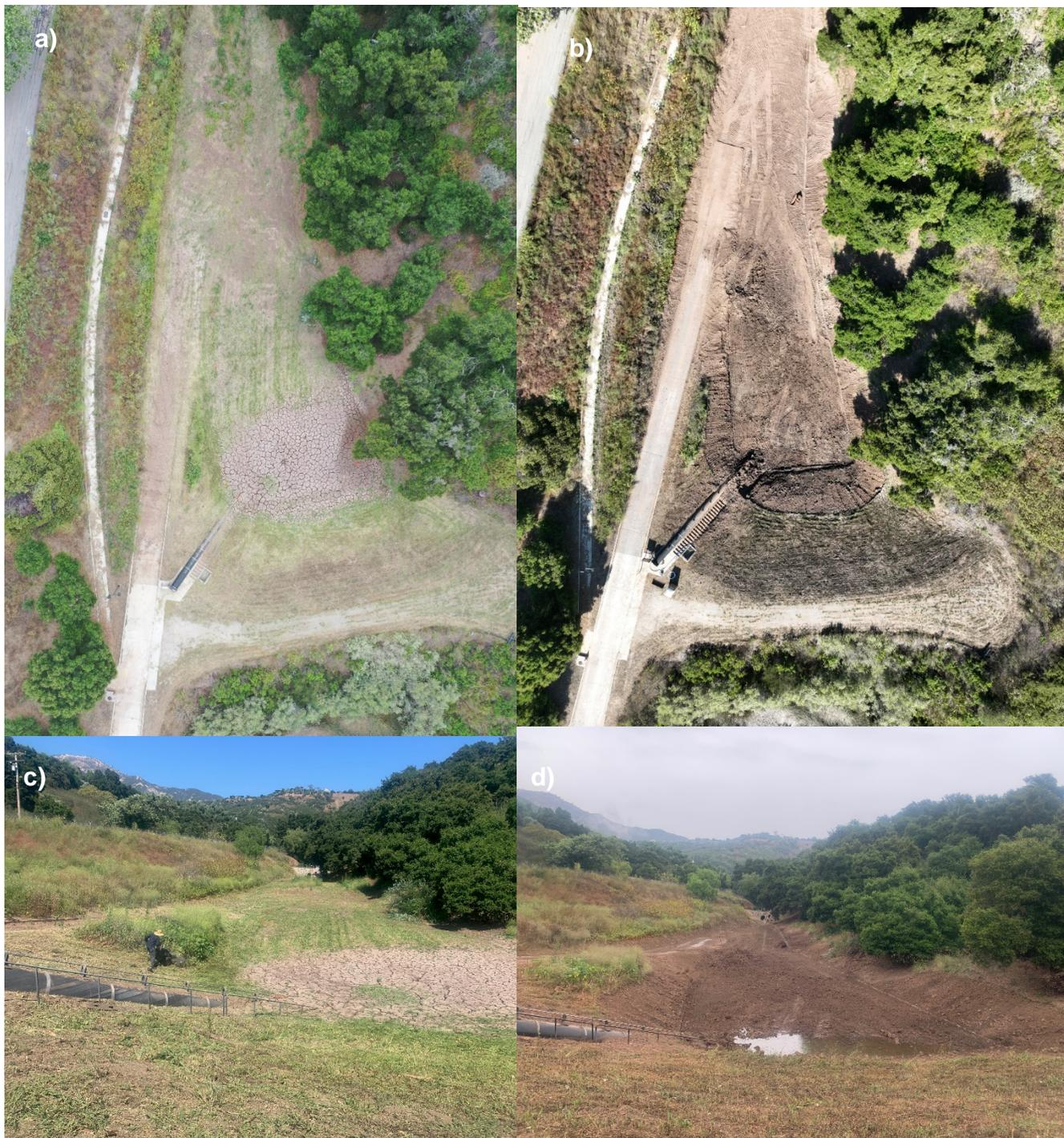
**Figure 1.** Lauro Debris Basin post-storm and de-watered, left (a), (c); post sediment removal, right (b), (d).
